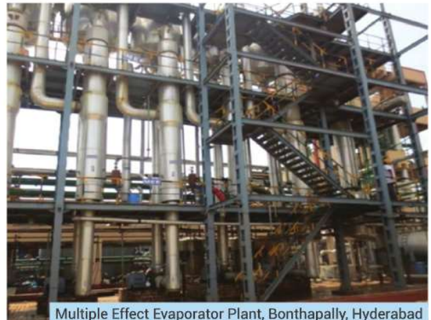
Multiple Effect Evaporator Plant, Bonthapally, Hyderabad
